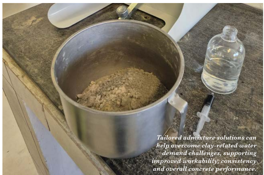
The Chryso Clear Test quantifies clay-admixture interactions to support optimal concrete mix design and improved performance consistency.
